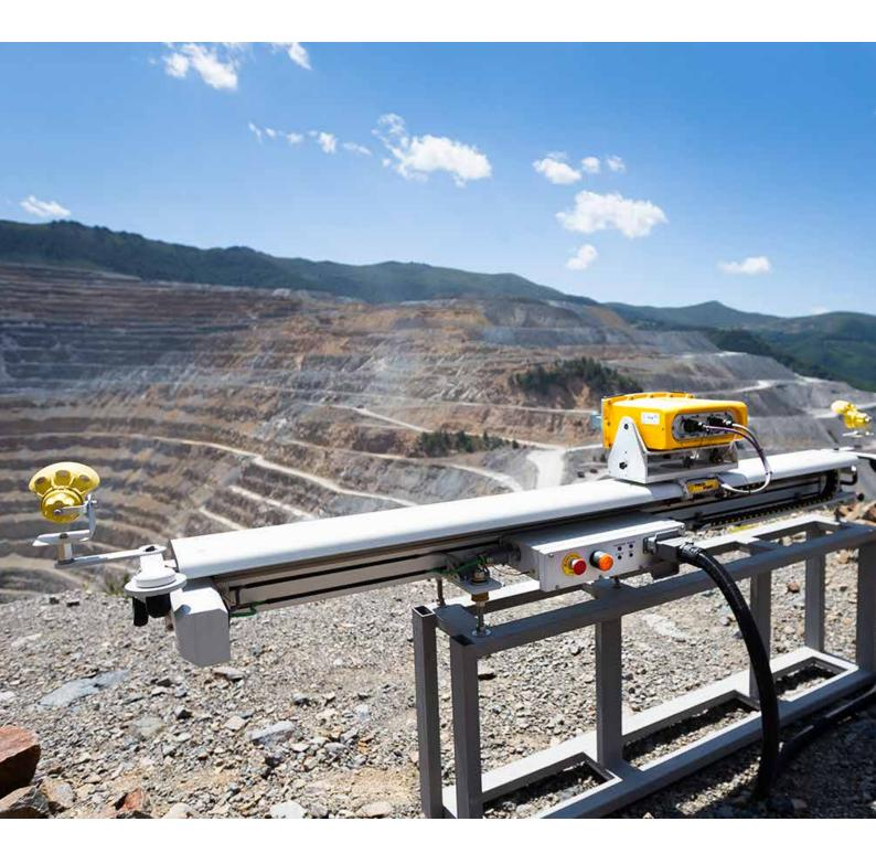
Next generation long-range radar for open-pit slope monitoring
